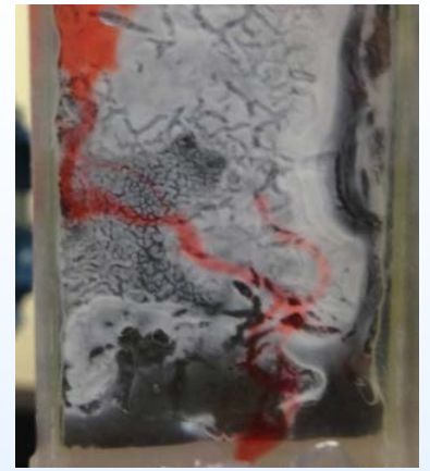
Brine (red) channeling through gelled polymer
